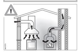
▶ Great care should be taken when using the cooker hood at the same time and in the same room or area of the house as another heating appliance which depends on the air in the room. Such appliances include gas, oil, wood or coal-fired boilers and heaters, continuous flow or other water heaters, gas hobs, cookers or ovens which draw air in from the room and duct exhaust gases out through a chimney or extraction ducting. When used in extraction mode, the
